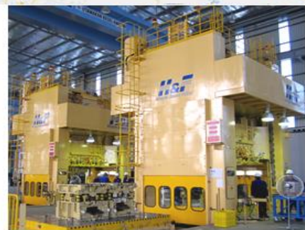
1000Ton-600Ton Tandem Press UNIPRES CORPORATION
